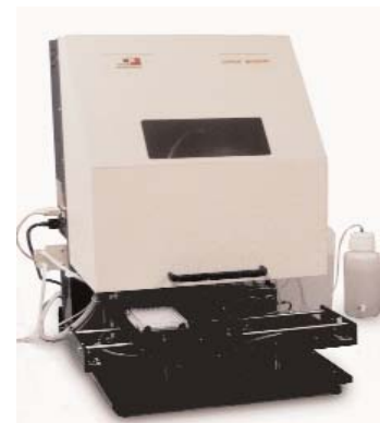
Figure 1. The COPAS BIOSORT was used to dispense 3,000 Cl.elegans of a certain stage into a tube in 8 minutes.
